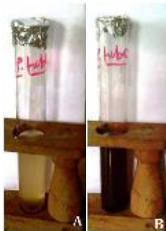
Figure 1: (A) Photograph of P. tuber-regium extract and (B) AgNO 3 and P. tuber-regium extract mediated silver nano particle solution after 2hours of incubation at 80 °C.
